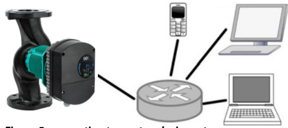
Figure 5: connecting to a network via router
